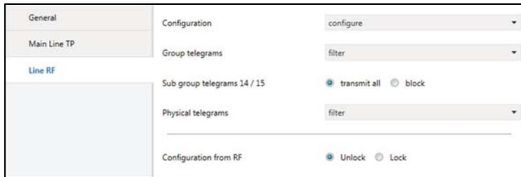
Picture 5 Funklinie Fenster / Line RF Window
